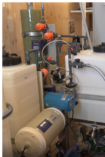
Figure 5: Hybrid FO-RO pilot plant with 140 L/h permeate production capacity
