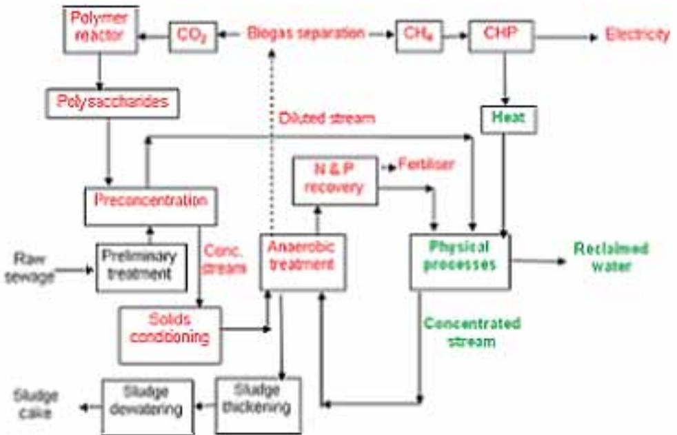
**Figure Schematic diagram of a possible 2030 wastewater treatment anaerobic flow sheet (GWRC, 2010)**
